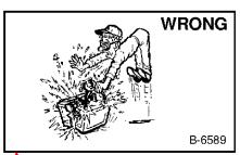
Lead-acid batteries produce flammable and explosive gases.
