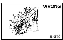
Lead-acid batteries produce flammable and explosive gases.
