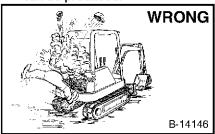
Stop, cool and clean engine of before flammable materials checking fluids.
