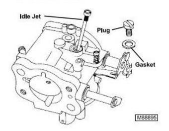
Install idle jet, plug and gasket. Tighten plug securely.
