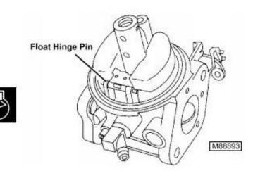
11. Install float hinge pin into place.
