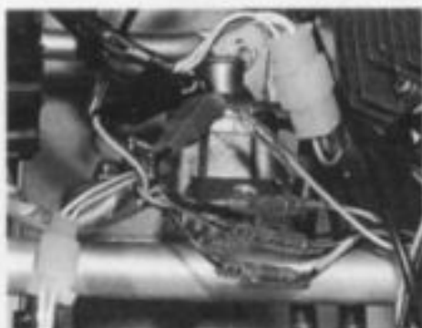
4.11a Disconnect generator wiring from main wiring loom - TZR125 shown
