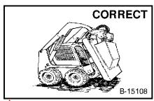
Always install approved lift arm support device when servicing rotary cutter. Raise lift arms and tilt Bob-Tach fully forward.
