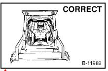
Always use the seat bar and fasten seat belt snugly. Always keep feet on the pedals when operating loader.
