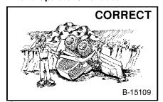
Always check work area before operating rotary cutter. Never use loader without operator cab with ROPS and FOPS approval. Fasten your seat
