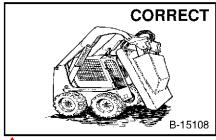
Always install approved lift arm support device when servicing rotary cutter. Raise lift arm(s) and tilt Bob-Tach fully forward.
