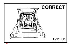
Always use the seat bar and fasten seat belt snugly. Always keep hands and feet on the controls when operating machine
