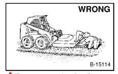
not put hands, feet, or objects under rotary cutter when engine is running.
