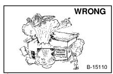
Do not use machine or rotary cutter in atmosphere with explosive dust, explosive gas, or exhaust where contact can flammable material.
