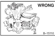
Do not use loader or rotary cutter in atmosphere with explosive dust or gas or where exhaust can contact flammable material.
