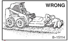
Do not put hands, feet or objects under rotary cutter when engine is running.
