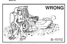
Keep bystanders away when operating rotary cutter. Do not operate without blade shut-off device.
