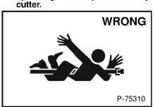
PTO master Keep shield. implement shield, and driveline quards in place.
