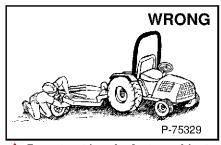
Do not put hands, feet, or objects under three-point rotary cutter when engine is running.
