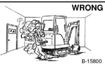
Vent exhaust to outside when engine must be run for service. Exhaust system must be tightly
