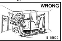
Always lower the bucket and blade to the ground before doing anv maintenance.
