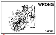
batteries Lead-acid produce flammable and explosive gases.
