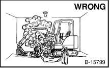
Have good ventilation when weldina or grinding painted parts.
