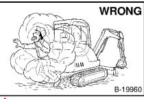
Vent exhaust to outside when engine must be run for service.
