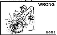
Lead-acid batteries produce flammable and explosive gases.
