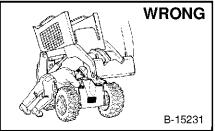
Disconnecting or loosening any hydraulic tubeline, hose, fitting, component or a part failure can cause lift arms to drop. Do not go under lift arms when raised unless supported by an approved lift arm support device. Replace it if damaged.
