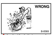
Lead-acid batteries produce flammable and explosive gases.
