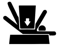
If you must work on a lifted machine or attachment, securely support the machine or attachment.
