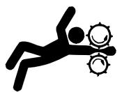
Tie long hair behind your head. Do not wear a necktie, scarf, loose clothing, or necklace when you work near machine tools or moving parts. If these items were to get caught, severe injury could result.
