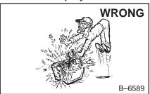
produce Lead-acid batteries flammable and explosive gases.
