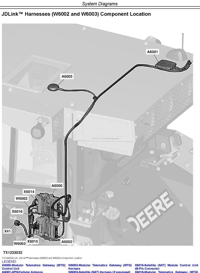
A6001-GPS/Cellular Antenna A6002-Satellite (SAT) Module Control Unit (if equipped) A6003-Satellite (SAT) Antenna (if equipped) JDLink is a trademark of Deere & Company
