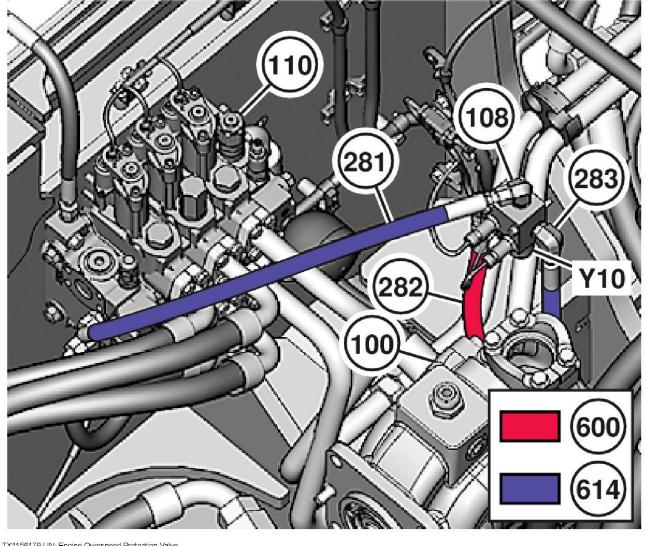
TX1156179-UN: Engine Overspeed Protection Valve LEGEND:
