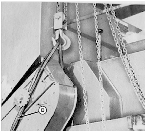
YC0680-UN: Attaching Lifting Strap
