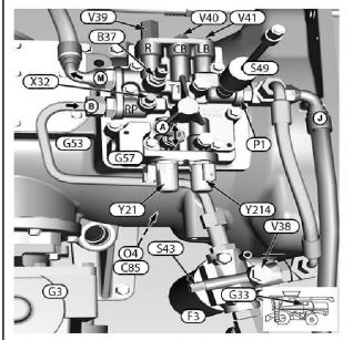
H122135-UN: G57 - Main Gearcase Valve Block - Three Speed and Push Button Shift Transmission
