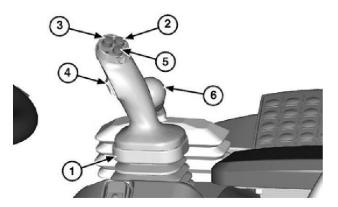
Joystick Bucket and Boom Control with Gearshift, Quick Shift Switch, FNR Switch, and Third Function Auxiliary Control Lever
