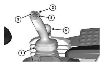
Joystick Bucket and Boom Control with Gearshift, Quick Shift Switch, and Third Function Auxiliary Control Lever
