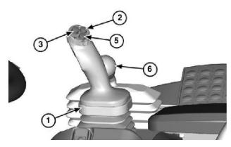
Joystick Bucket and Boom Control With Gearshift, Quick Shift Switch, and Third Function Auxiliary Control Lever
