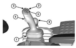
Joystick Bucket and Boom Control With Gearshift, Quick Shift Switch, FNR Switch, and Third Function Auxiliary Control Lever
