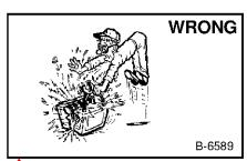
Lead-acid batteries produce flammable and explosive gases.
