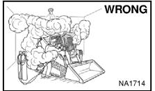
Have good ventilation when welding or grinding painted parts.
