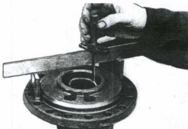
Fig. 21—Measure distance between right axle housing flange and bearing cup seat (shoulder).
