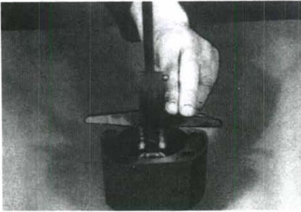
Fig. 42—Using a depth gage, measure distance between outer and inner faces of right side rod guide. Refer to text.
