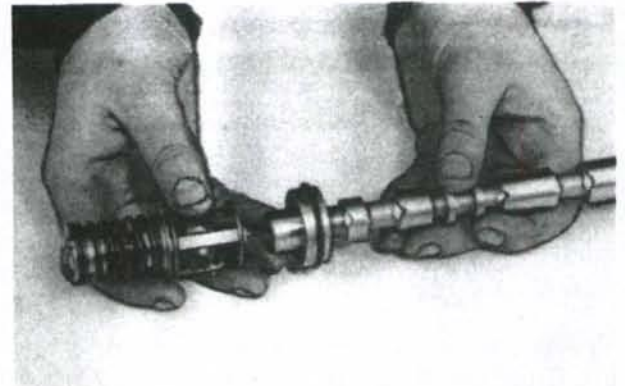
Fig. 173—View of detent assembly removed from valve spool. Do not disassemble detent unit as no parts are available.
