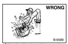
Lead-acid batteries produce flammable and explosive gases.
