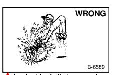
Lead-acid batteries produce flammable and explosive gases.
