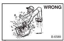
Lead-acid batteries produce flammable and explosive gases.
