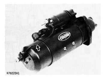
Fig. 2-Solenoid Ground Wire (8630 Tractor Only)
