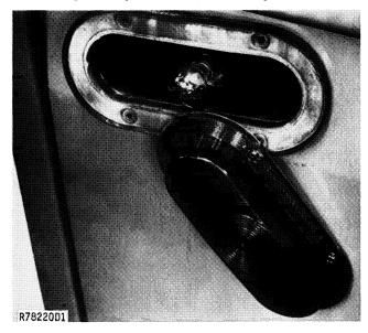
Fig. 25-Removing Tail Lamp Bulb
