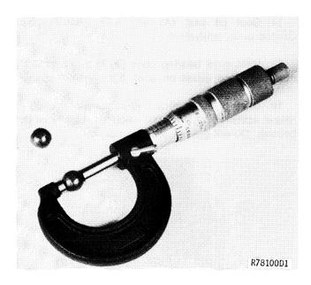
Fig. 19-Checking Lead Ball Size
