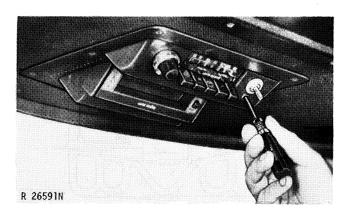
Fig. 15-Adjusting Antenna Trimmer Capacitor Screw on Motorola Radio
