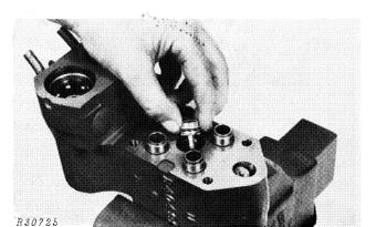
Fig. 15-Flow Control Valve Stop Installation - Later Model
