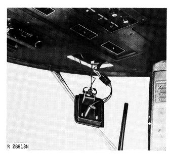
Fig. 30-Removing Console Lamp Bulb
