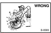
Lead-acid batteries produce flammable and explosive gases.
