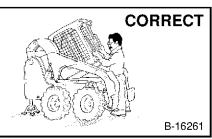
Lise the correct procedure to lift or lower operator cab.
