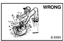
Lead-acid batteries produce flammable and explosive gases.
