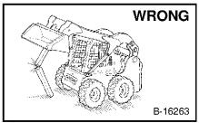
Never work on loader with lift arms up unless lift arms are held by an approved lift arm support device. Replace if damaged.
