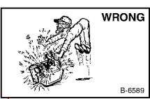
Lead-acid batteries produce flammable and explosive gases.
