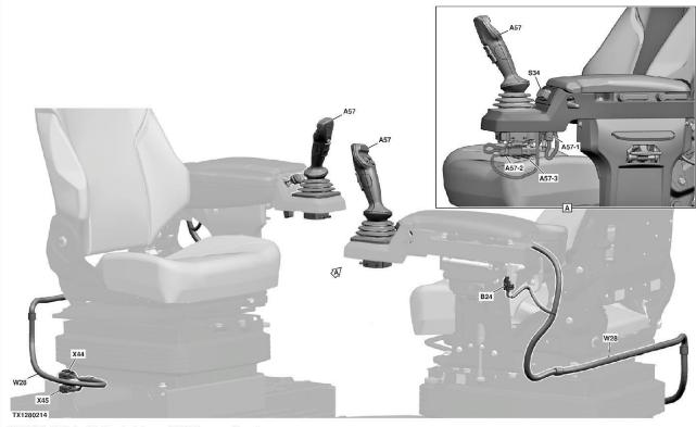
TX1280214-UN: Joystick Steering Harness (W28) Component Location
