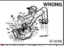
Lead-acid batteries produce flammable and explosive gases.
