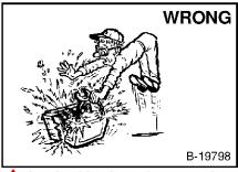
Lead-acid batteries produce flammable and explosive gases.
