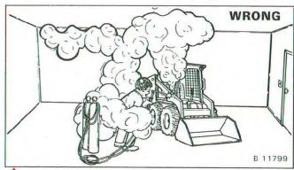
Have good ventilation when welding or grinding painted parts. Wear dust mask when grinding painted parts. Toxic dust and gas can be produced.
