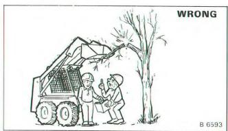
Never work on loader with lift arms up unless lift arms are held by a lift arm support device.
