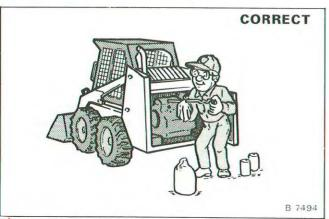
Keep rear door closed except for service. Close and latch door before operating the loader.
