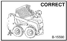
Lise the correct procedure to lift or lower operator cab.
