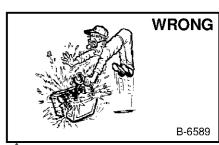
Lead-acid batteries produce flammable and explosive gases.
