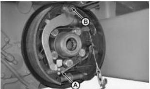
Parking brake cable Remove parking brake cable (A).
