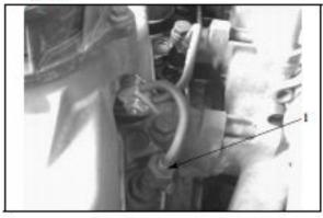
Fit Adapter D2 to the nozzle holder mounting, and connect with gauge assembly
