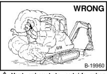
Vent exhaust to outside when engine must be run for service. Exhaust system must be tightly sealed. Exhaust fumes can kill without warning.
