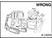
Keep body, jewelry and clothing away from moving parts, electrical contact, hot parts and exhaust.
