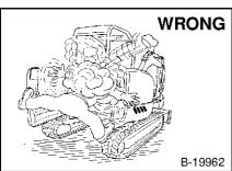
Stop, cool and clean engine of flammable materials before checking fluids.
