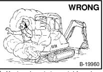
Always lower the bucket and blade to the ground before doing any maintenance. Never modify equipment or add
