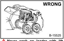
Never work on loader with lift arms up unless lift arms are held by an approved lift arm support device. Replace if damaged.
