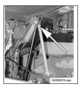
Set the lever at the pump to "pump down" and pump the cab downward until the safety rod is secure against the right side of the cab floor.
