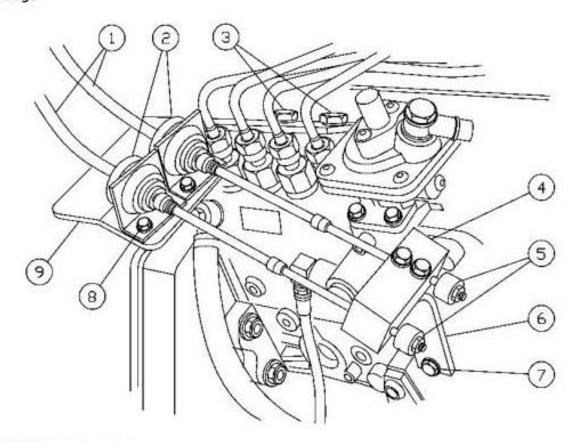
Dual Throttle Linkage at engine
