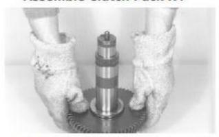
Heat Gear and Install
