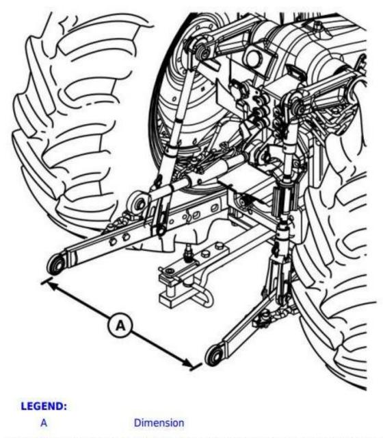
Adjust both turnbuckles equally to achieve specified dimension between insides of draft link balls.
