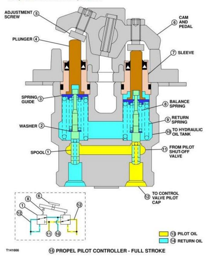
Propel Pilot Controller-Full Stroke
