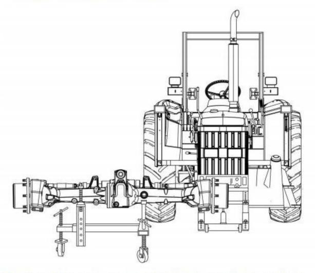
[1] - Raise tractor and support safely using JT05725 Universal Support Stand and/or a suitable lifting device.
