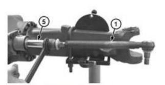
Tie Rod From Piston Rod Removal Remove tie rod (1) from steering cylinder piston rod (5).
