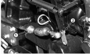
Throttle Cable-To-Injection Pump Connection
