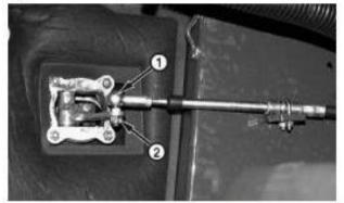
Throttle Cable-To-Accelerator Pedal Connection
