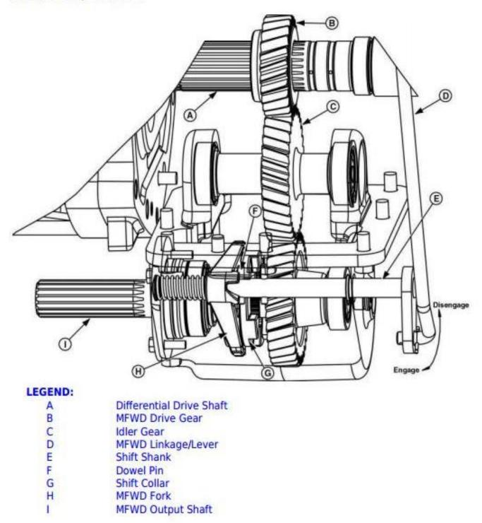
The main function of the MFWD gearbox system is to provide power to the front axle when added traction is necessary.
