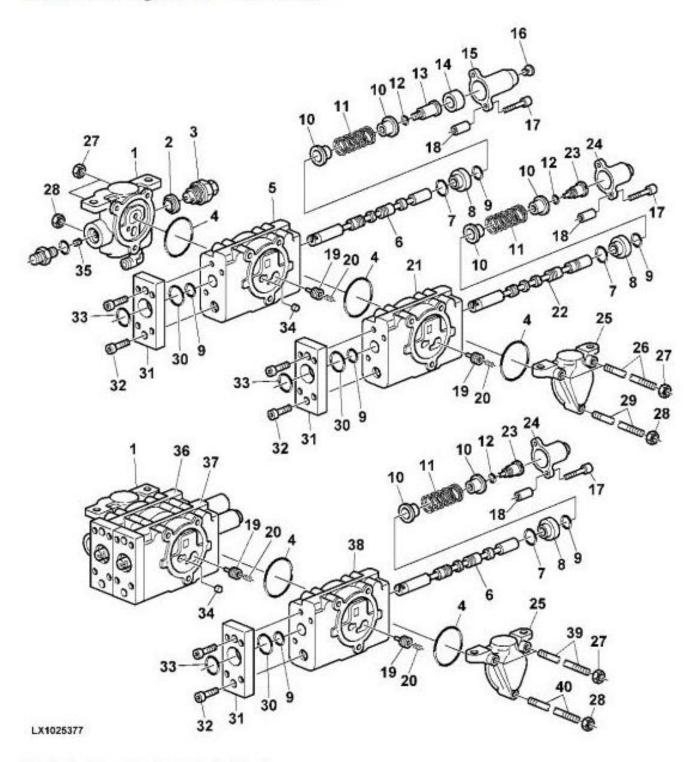
Control valves (electrical actuation)
